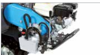
Lever-operated hydraulic tipping control valve.
