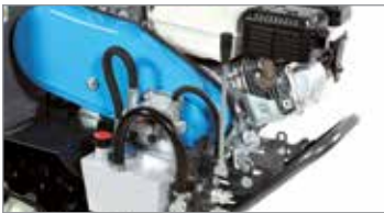
Lever-operated hydraulic tipping control valve.
