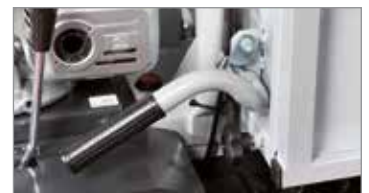
Manual dump with automatic locking system.
