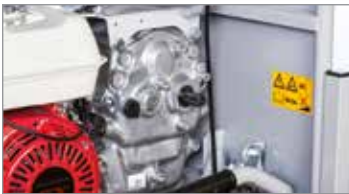
Independent PTO at 2100 rpm.
