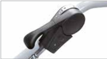
Handlebar-mounted PTO control.
