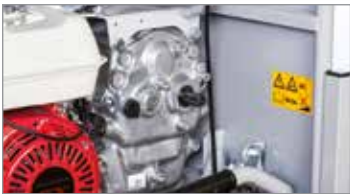
Independent PTO at 2100 rpm.
