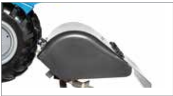
50 cm wide counter-rotating rotor to facilitate work on particularly difficult terrain.
