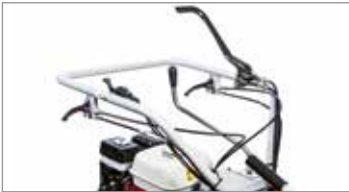
Steering with independently controlled releases and brakes.
