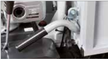
Manual dump with automatic locking system.
