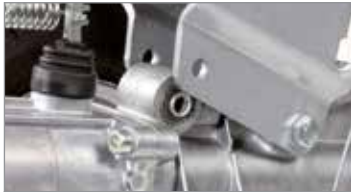
Handlebar mounted on vibration dampers.
